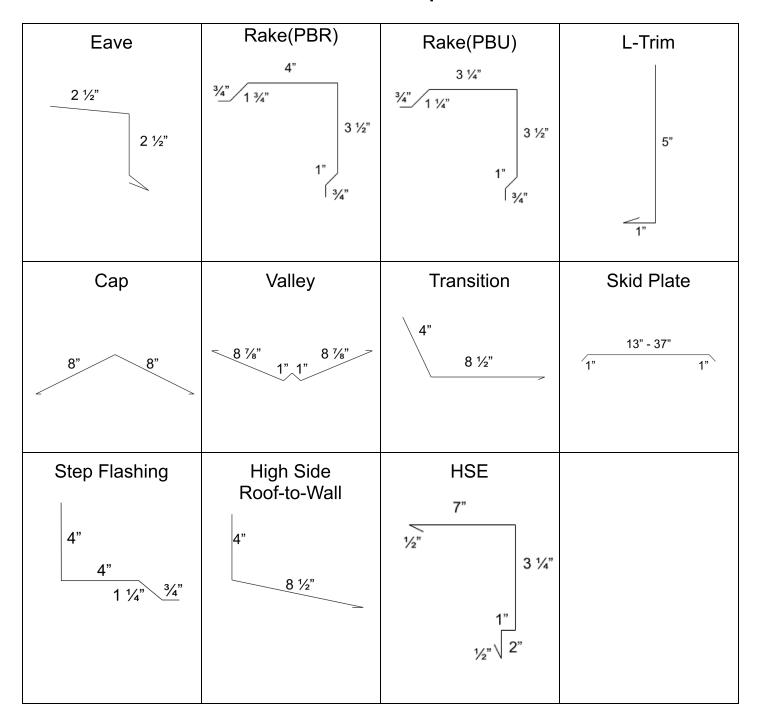
These standard trim diagrams are for customer reference and can be altered to jobsite specifications. All trim components produced by St Martin Metal are made using 26 gauge, 50 grade, pre-painted steel material. Custom trim components can be made to order. All trim components are produced in sections being 10' 1" in length, however trim components can be specially ordered in lengths up to 20', with a lead time of 6-8 business days.
